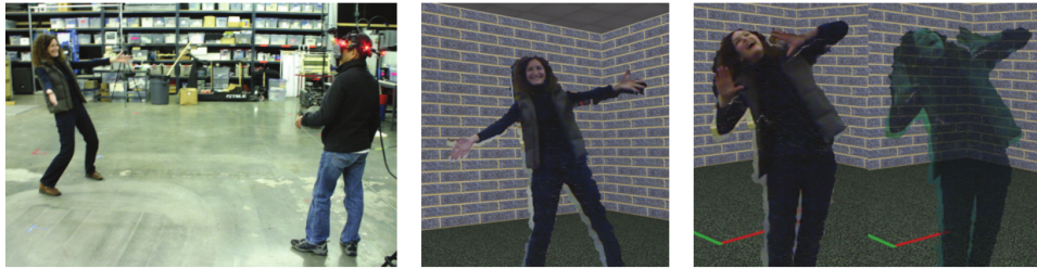
Figure 3: from left to right: a person in the real world environment of the user, the segmented person rendered in the virtual environment, use of different rendering techniques to achieve a hologram effect [SKB11]
