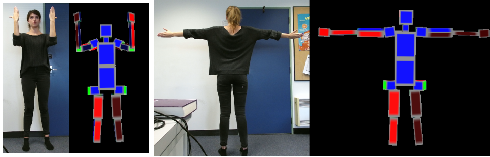
(a) Rotation of fore arm can be detected. (b) No distinction between front and back side of the user is possible.
