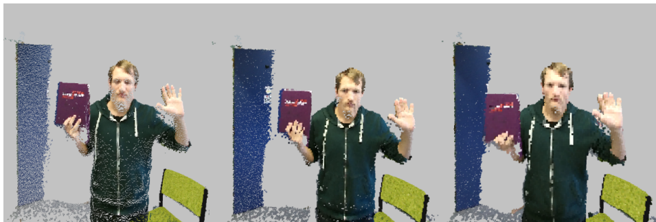
Figure 18: result of different voxel sizes from left 0.5cm, 0.8cm, 1cm, the smaller voxel sizes preserve more details, especially noticeable at the hands and the face, but introducing missing voxel due to oversampling the Kinect data
