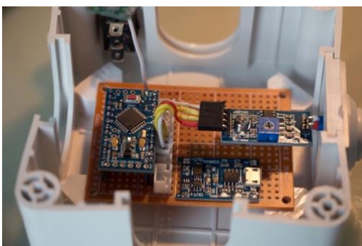
Figure 3. 22 Soil Moisture Sensor Mounted (own illustration)
