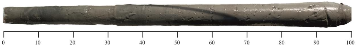
Figure 7. Freeze core obtained with a freezing lance (dimensions in cm).
