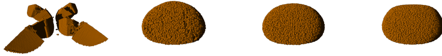
Figure 18: Numerical fracture on a hyperelastic (Neo Hookean) sphere sampled at one particle per cell. From left to right: grid, random, stratified and poisson disk sampling.
