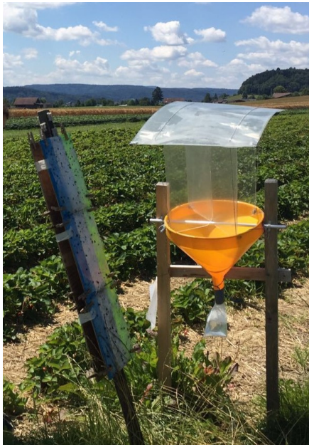
S2 Fig. Sampling point with the two trap types. The combi trap (yellow, 42.5 cm upper diameter) has a whirl-pack® bag (Sigma-Aldrich) attached on the bottom, filled with 95% ethanol and a roof on top to prevent dilution through rain. For the sticky trap (891cm x 210cm), foils (Folex Foils Laserptinter BG-64 from OfficeWorld Switzerland) are attached with clothes pegs and/or tape to the coloured board (yellow, blue, white; Sparvar UV reflecting colour of Spray-Color GmbH) and were then sprayed with glue (Soveurode spray glue from Witasek, Austria).
