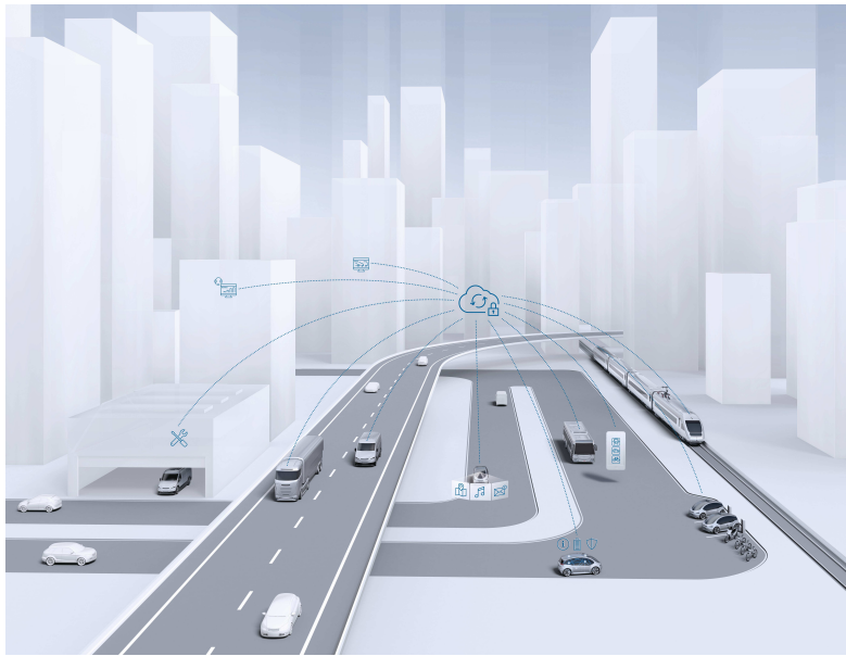
Figure 2.1: Illustration of an intelligent transportation system. Vehicles are able to exchange information with each other and an infrastructure in order to harmonize the operation of vehicles (source: Bosch Mediaspace [24]).
