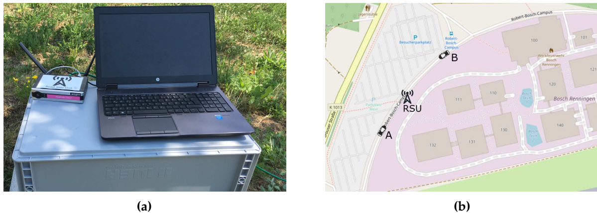
Figure 5.28: Functional tests of the prototype: (a) Illustration of a RSU deployment at the road side. For measurement purposes, a laptop PC is used to monitor the traffic flows. (b) The testbed deployed next to the Bosch research campus in Renningen, Germany.
