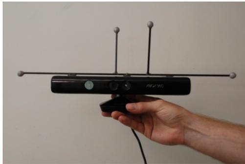
**Figure 5.1:** This figure shows a handheld Kinect RGB-D camera with attached motion capture markers used during the recording of the dataset. The markers are tracked by a motion capture setup for ground truth [SEE<sup>+</sup>12].
