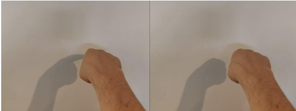
Figure 8 Index finger tracking issue. Only the shadow makes it clear whether a finger is extended or not
