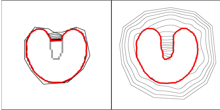
Figure 3.6: Convergence comparison: Snake (left) vs Snake with GVF. The red color shows the final segmentation.
