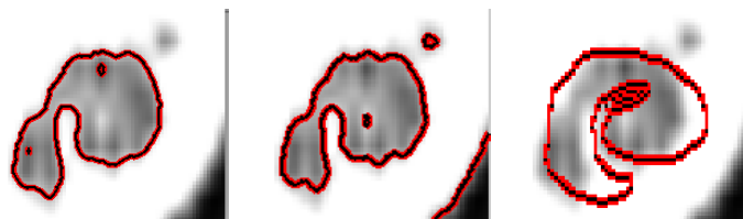
Figure 4.7: Sample of the results of the CT images, from left to right: Chan-Vese, GAC and ASM.
