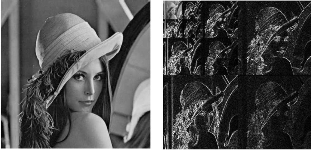
**Figure 3.2:** Example of a three level Wavelet decomposition of an image with Haar basis [Nie07]
